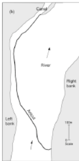
Figure 1 Irregularly shaped traditional anicut. Scale in meters.
