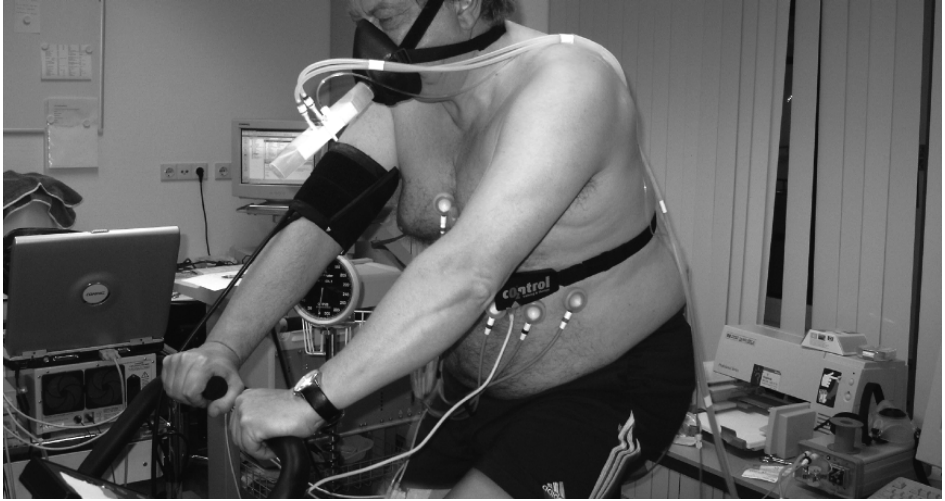
Fig 1. Experimental setup to assess maximum heart rate, peak oxygen uptake and maximum workload capacity of our patients during a ECG-stress test on a cycle ergometer.
