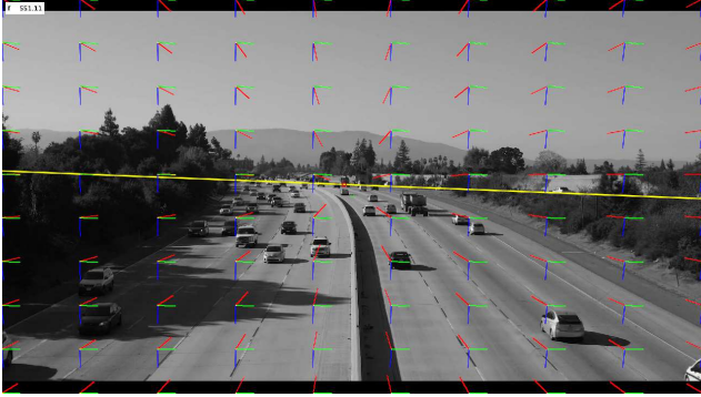
Figure 1. Illustration of three orthogonal vanishing points detected in a highway scene.
