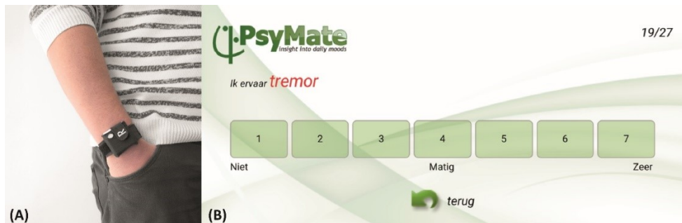
Figure 1. Recording modalities. a Wearable sensor attached to the wrist via a wristband. b Screenshot of the question ‘Ik ervaar tremor’ (‘I experience tremor’) on a 7 point Likert scale, with a score of 1 indicating not at all and a score of 7 indicating very much.
