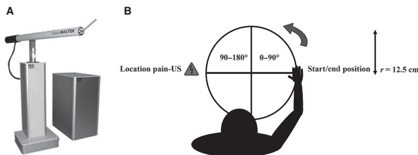
**Figure 1** Overview of the HapticMaster (A) and one of the circular movements (B; a counterclockwise movement). During CS+ acquisition trials, the pain-US was administered when the hand crossed at 180° of the movement.
