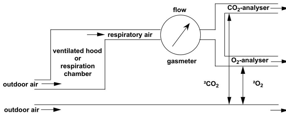
**Figure 1** Schematic representation of an open-circuit system for the measurement of oxygen consumption and carbon dioxide production as applied in a ventilated hood and a respiration chamber.
