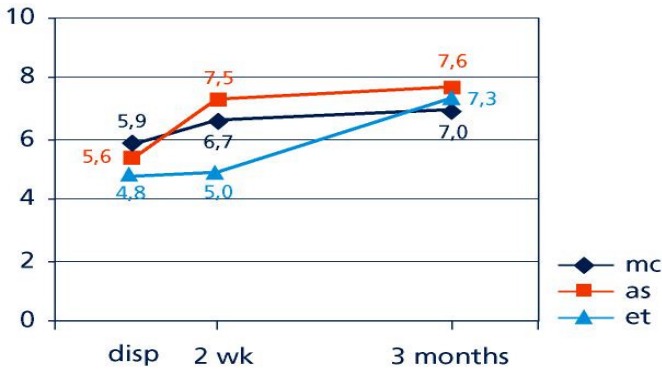
FIGURE 5. Comfort scores for a multicurve (MC), aspheric (AS) and edge toric (ET) lens design.
