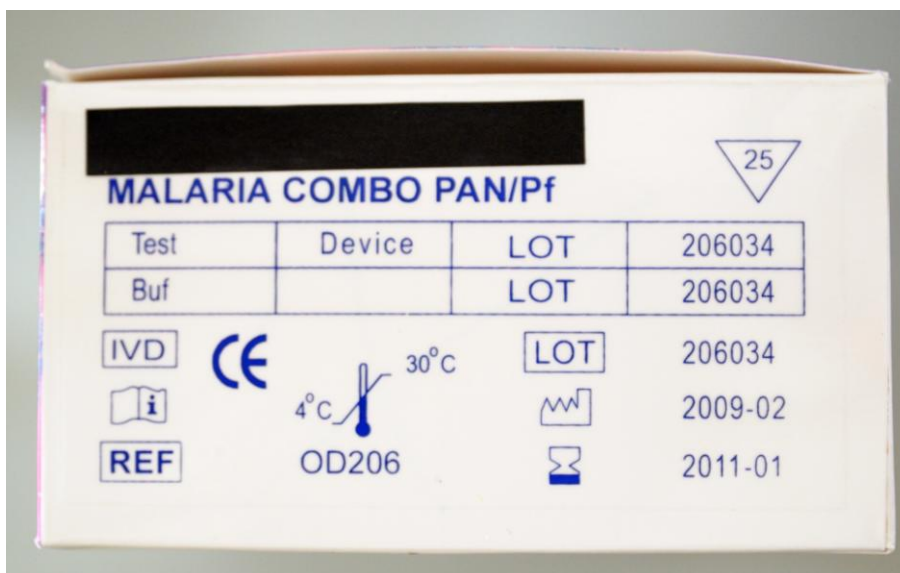
Figure 12: Example of the lateral side of a RDT box: all essential information is printed on a single side of the box, contributing to clear storage. Of note, the symbol used for “sufficient for” is not used as required by EN 980: the inverted triangle should contain the “Σ” character and affix the number below of beneath.
