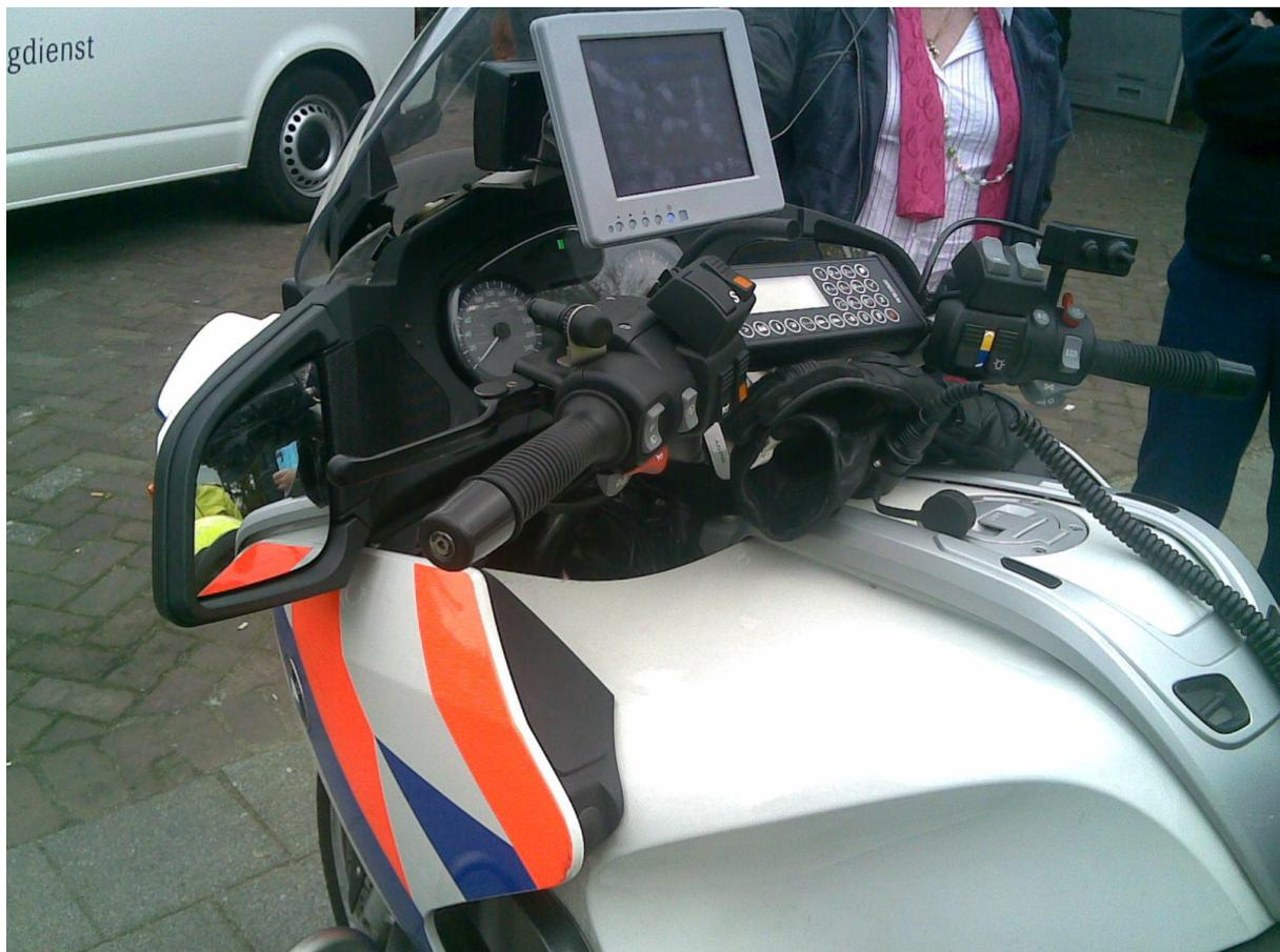
**Figure 7** – A mobile unit of the Dutch police equipped with ANPR hardware and software. The bigger screen displays real-time information of ANPR hits.
