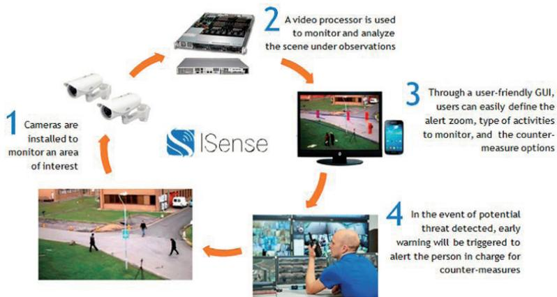
Figure 9.2: iRadar's iSense™ Smart Video Surveillance System
