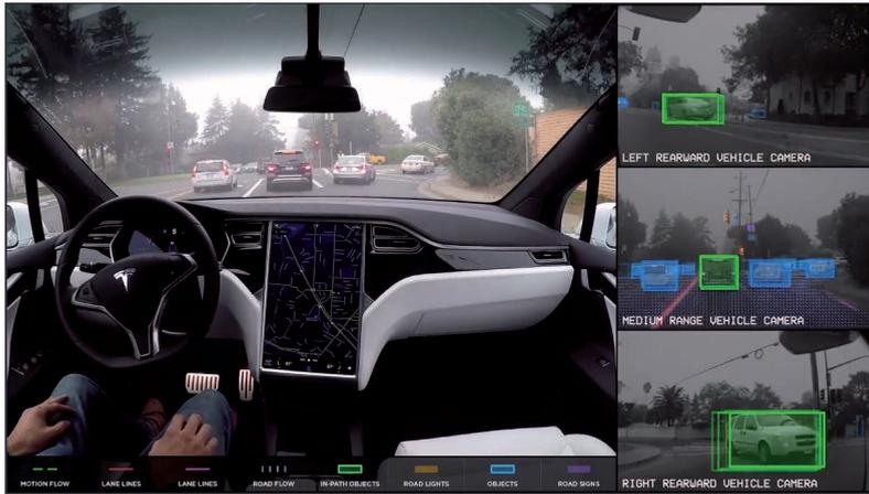
Figure 9.1: Object detection and recognition helps for understanding the environment in autonomous navigation: a snapshot of the vision system of Tesla Autopilot in driving <sup>1</sup>.
