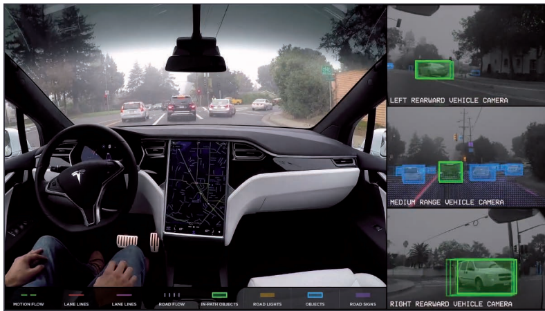
Figure 9.1: Object detection and recognition helps for understanding the environment in autonomous navigation: a snapshot of the vision system of Tesla Autopilot in driving 1 .
