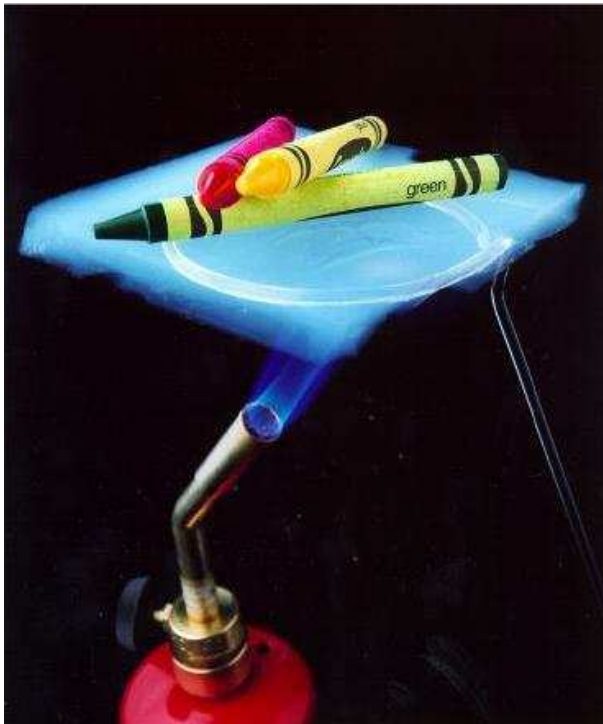
Figure 3: Crayons supported on an aerogel over a flame
