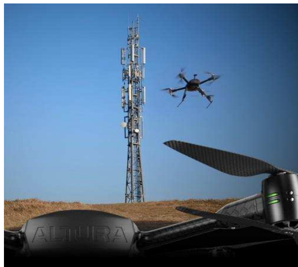
Aerialtronics Altura Rotorcopter for site inspection
