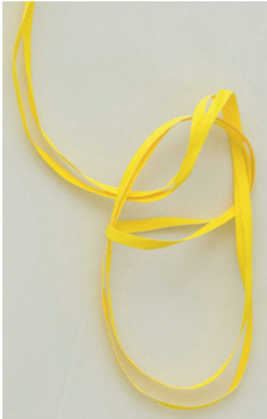
Figure 1. 4 mm-wide radiopaque UHMWPE sublaminar wire and the double loop sliding knot with extra pass used to secure the wire.
