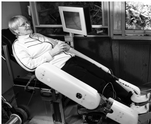
Figure 7.3 The MoreGait is a pneumatically actuated robot for the training of ambulatory function. The device allows the use at the patient's home.
