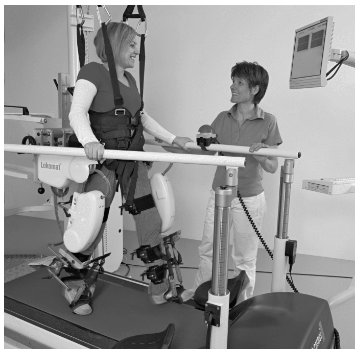
Figure 9.1 The Lokomat is an actuated robotic exoskeleton for the training of ambulatory function on a moving treadmill. The patient is secured by an overhead suspension system which partially relieves the body weight. Position sensors and force transducers are used to monitor the efforts of the patient (Picture by courtesy of Hocoma AG).
