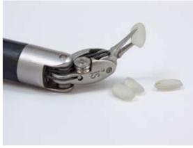
Figure 9. The specially designed robotic instrument tips offer six degrees of freedom and allow for intuitive manipulation.
