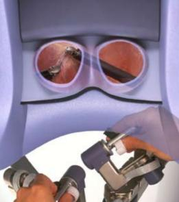
Figure 2. The tips of the instruments are projected on the location where the finger tips of the surgeon are, allowing optimal restoration of the eye-hand-target axis. The controls allow for a natural forceps-like grip.
