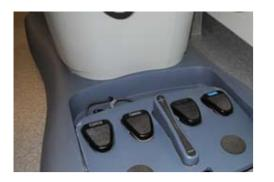
Figure 5. The console holds a number of foot pedals, allowing for adjustments of the manipulating and visual systems.
