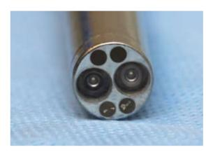
instruments adjusted to the patient side cart. A double-channel stereoscopic 12mm videoendoscope (Figure 3) contains two lenses approximately 8mm separate from each other. It generates two slightly different images that are transposed through two separate vision canals. After correcting the images for the mean inter papillary distance of 60mm, the images are sent to two separate High-Definition displays in the console.
