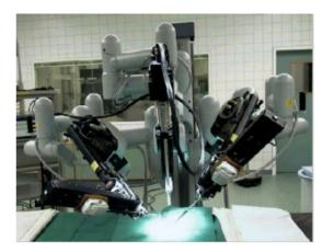
Figure 8. The patient-side cart holds one arm for the visual system and three arms for manipulation
