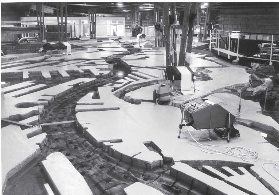
Figure 3.1 The Rijnmond model in operation. Note the devices used to register water levels located at various points of the model. © Deltares.
