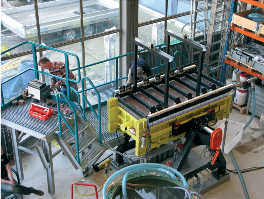
Figure 4.5 Model used during medium-scale piping experiments. The model is shown without the plastic cover mentioned in the text. Photo by Vera van Beek. © Deltares.
