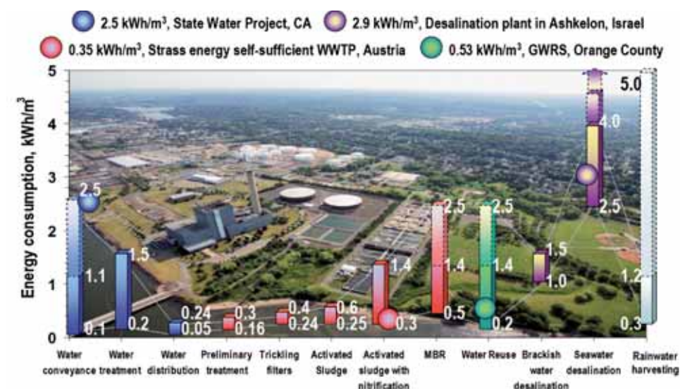
Figure 2: Typical energy footprint of the major elements and processes in water cycle management (Adapted from Meda and Cornel, 2010, Wilson, 2009, Voutchkov, 2010 and Lazarova et al, 2012).
