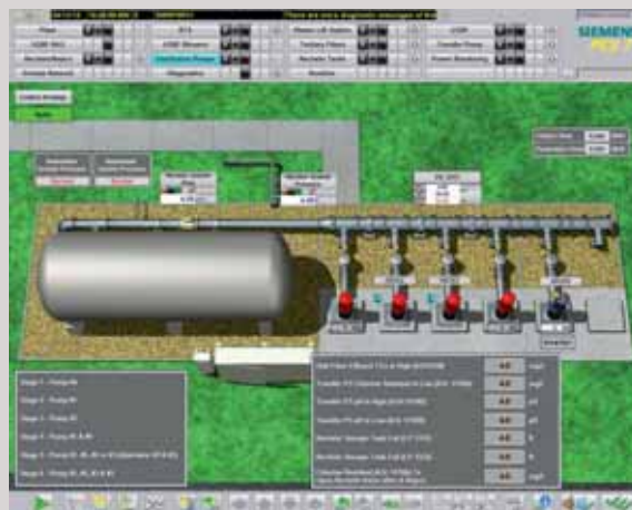
A screen shot from Volusia's plant control system which shows the status of the distribution pumps, and through which an operator can set up automatic control conditions for the pumps.
