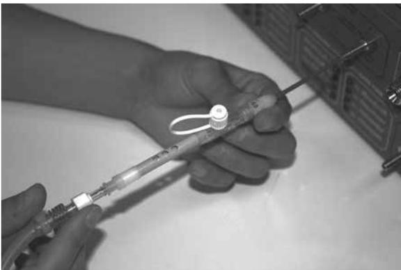
**Figure 2** The oxygen flow modulator connected to a transtracheal catheter with all five openings released during measurements in the experimental setting. In the shadow the two openings at the bottom of the device can be seen.
