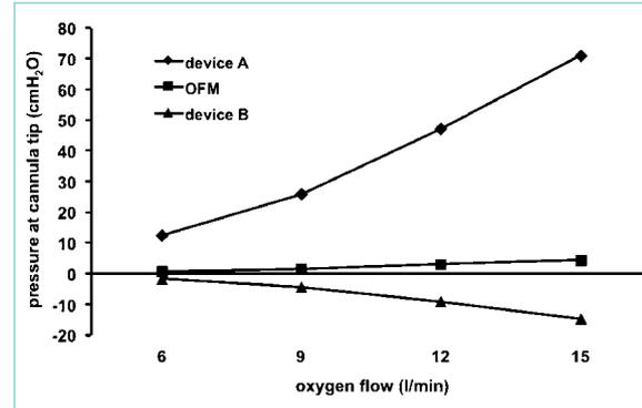
**Figure 4** Pressures measured at the tip of the 2-mm ID transtracheal catheter with different oxygen flows in device A (consisting of a 2-mm ID standard three-way stopcock connected in-line to the transtracheal catheter), device B (the transtracheal catheter connected to the side port of the 2-mm ID standard three-way stopcock) and the Oxygen Flow Modulator with all five holes open.
