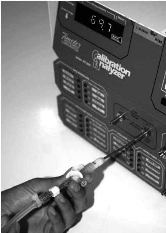
**Figure 1** Device A: a 2-mm ID standard three-way stopcock connected in-line to the 2-mm ID transtracheal catheter. The transtracheal catheter is tightly fitted into the orifice for low range positive pressure measurement of the monitor.
