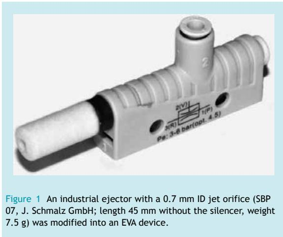
**Figure 1** An industrial ejector with a 0.7 mm ID jet orifice (SBP 07, J. Schmalz GmbH; length 45 mm without the silencer, weight 7.5 g) was modified into an EVA device.
