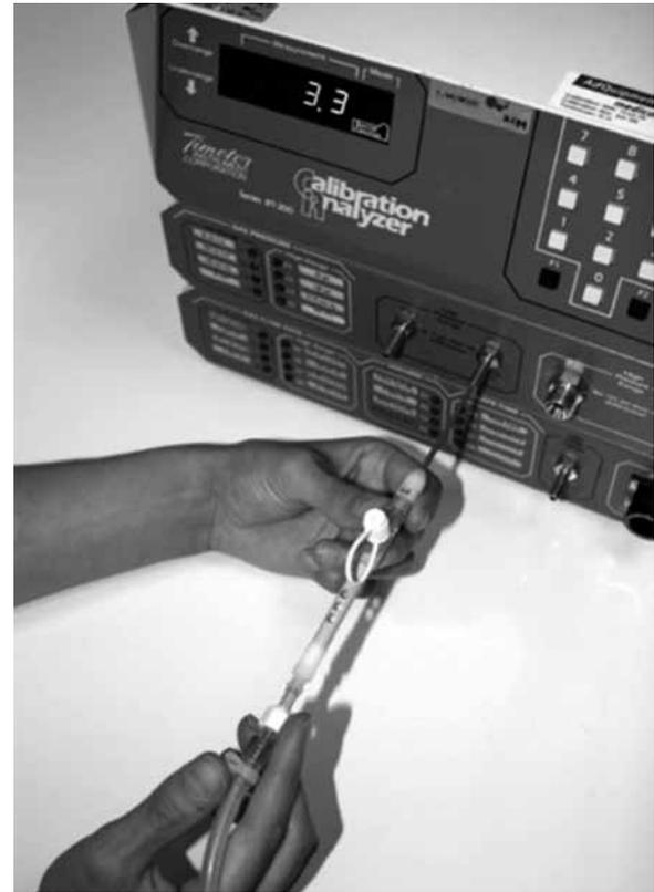
**Figure 3** The Oxygen Flow Modulator connected to the 2-mm ID transtracheal catheter with all five openings released during measurements in the first part of the experiments. In the shadow the two openings at the reverse side of the device can be seen.
