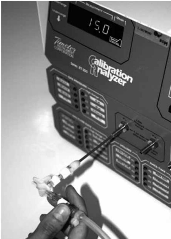
**Figure 2** Device B: a 2-mm ID standard three-way stopcock connected to the 2-mm ID transtracheal catheter via the side port. Note that the transtracheal catheter is put into the orifice for low range negative pressure measurement, thus the value indicates a negative pressure.
