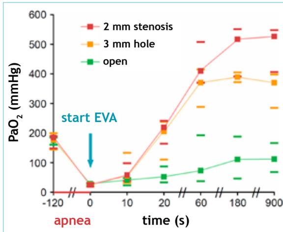
Figure 2A Course of  $PaO_2$  at different upper airway patency prior (-120 s) and after two minutes of apnoea (0) and subsequent EVA over 15 minutes (part 2 of the study). The ET was either fully open or obstructed with a 3 mm hole or a 50 mm long, 2 mm stenosis. Data presented as mean and range.
