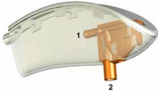
**Figure 1A** CAD model of the Ventrain. The shell is shown transparently, so the ejector as the functional centrepiece can be seen inside the shell. The oxygen tubing (not shown) is connected to the ejector's inlet (1) and short connecting tubing (not shown) is glued to the side port (2).
