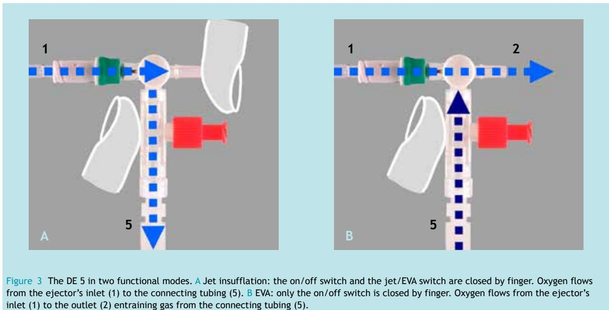
**Figure 3** The DE 5 in two functional modes. **A** Jet insufflation: the on/off switch and the jet/EVA switch are closed by finger. Oxygen flows from the ejector's inlet (1) to the connecting tubing (5). **B** EVA: only the on/off switch is closed by finger. Oxygen flows from the ejector's inlet (1) to the outlet (2) entraining gas from the connecting tubing (5).
