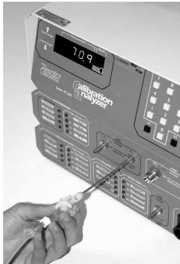
**Figure 3** Use of a conventional three-way stopcock (ID 2 mm) for emergency jet ventilation at a flow of 15 l·min<sup>-1</sup> results with the side port open in a pressure at the catheter tip of about 70 cmH<sub>2</sub>O.
