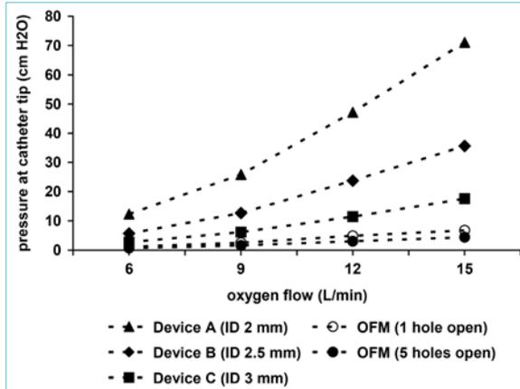
**Figure 4** Pressure measured at the tip of a 16 G and 13 G Ravussin needle and a 6 Fr transtracheal catheter using three self-assembled devices consisting of a three-way stopcock with different inner diameters (device A, B, and C) and the oxygen flow modulator.
