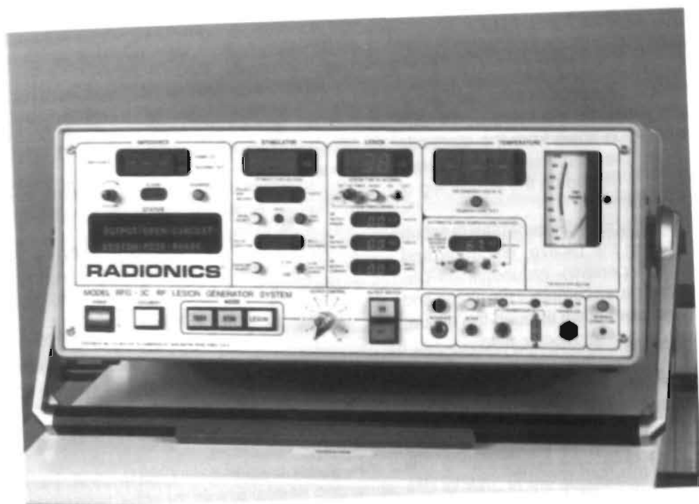
Figure 1. Radiofrequency lesion generator Radionics 3C with following functions: impedance monitor, stimulator, lesion parameters and temperature monitor.
