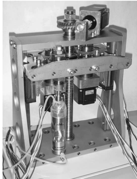
Fig. 2. Image of the bioreactor with one vessel installed.
