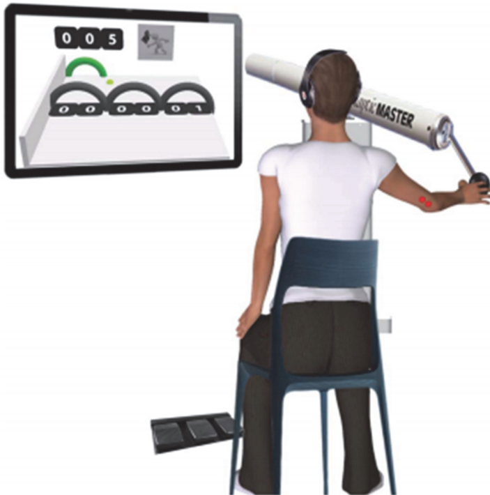
Figure 5.1. Experimental set-up showing the position of the participant in front of the screen, using the HapticMaster for the arm-reaching task.
