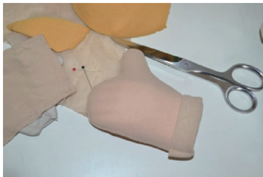
Figure 5.6 Creating KASPAR's thumb
