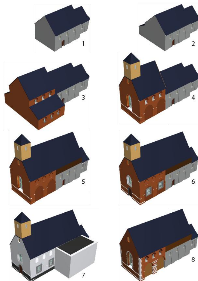
Figure 5-4: 3D models of the different building phases of Graethem chapel: (1) ca. 1120, (2) ca. 1230-45, (3) second half of the 13th century, (4) ca. 1500, (5) ca. 1658, (6) ca. 1720, (7) 19th century, (8) 20th century [Massart, 2014].
