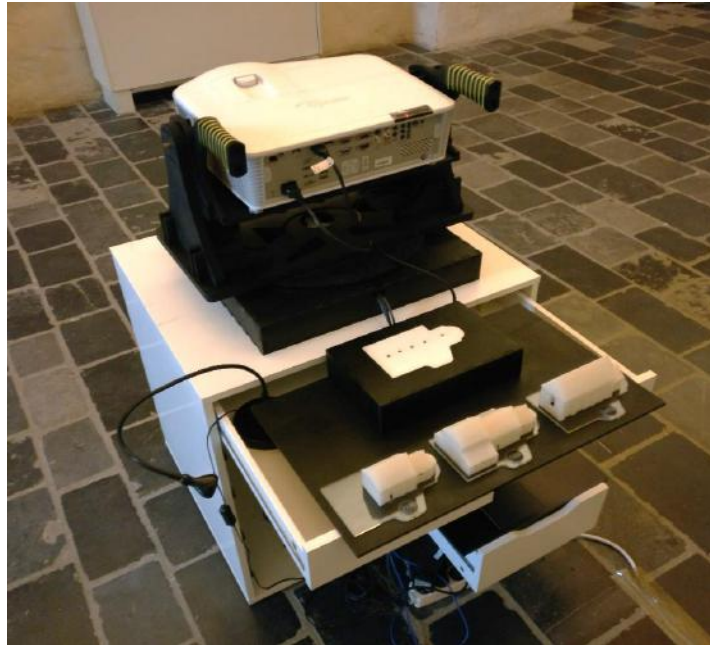
Figure 5-6: Final design of the installation: a freely rotatable projector combined with a tangible user interface (physical models of the chapel's building phases that visitors pick up and place them on the designated platform to activate the projection).
