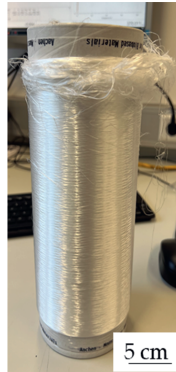
Figure 6.4: Broken filaments in bobbin
