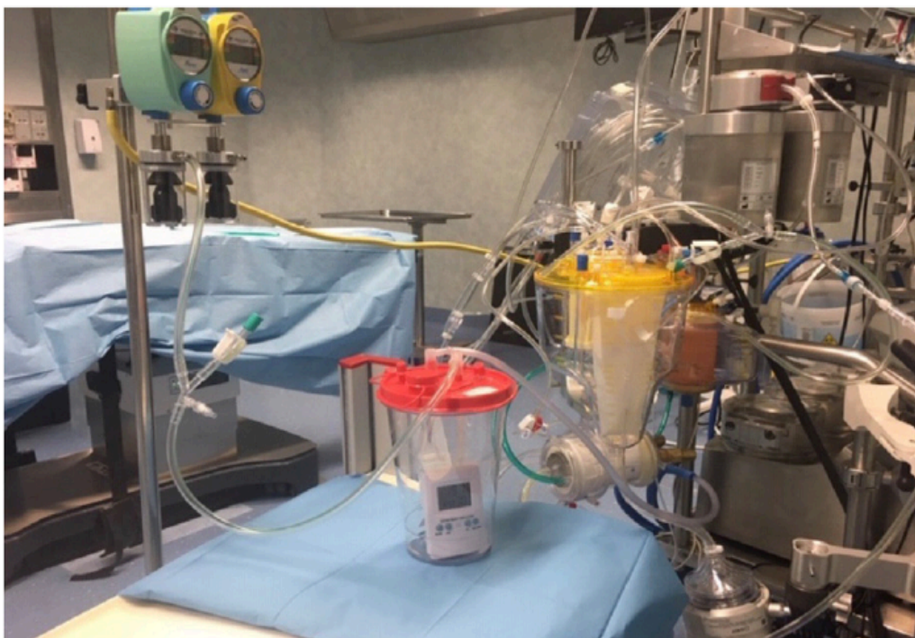
Figure 4. System for negative aspiration and measurement, which composes of four components:(1) retrofit tank of the heat exchanger for the accumulation of steam.
