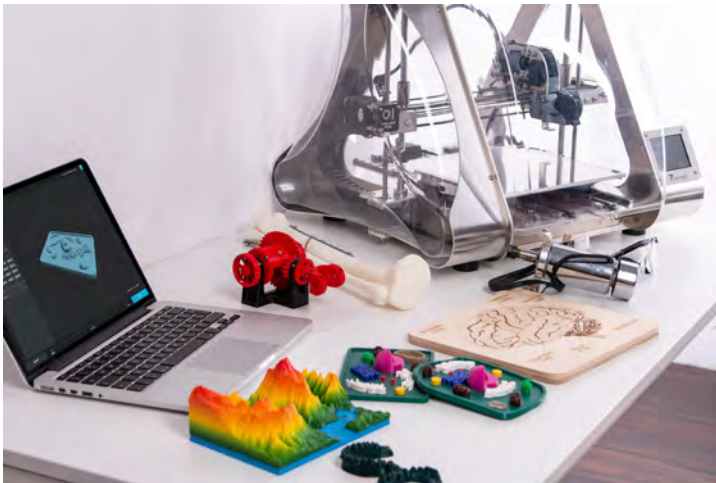
Figure 1.1: The prototyping revolution. A typical RP workstation including a computer with a CAD software and a slicing software, a prototyping tool and different materials. Adapted from zortrax.com
