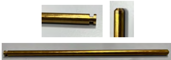
Figure S8. Brass rods used to guide the moving parts of the pump.
