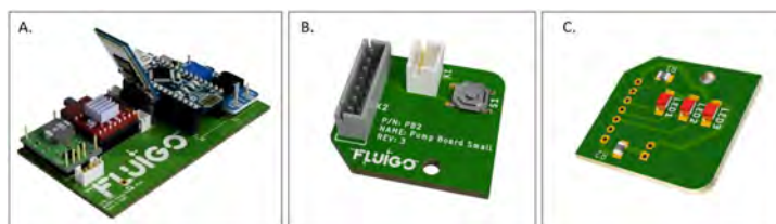
Figure 4.2: Electronic boards. A) Main board. B) Top layer of secondary board, C) bottom layer of secondary board
