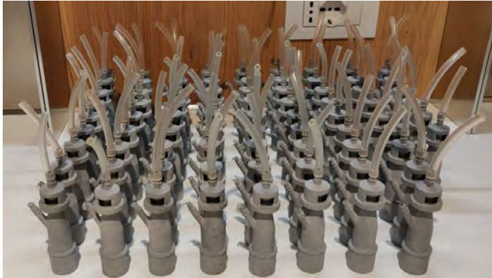
Figure 1.9: Rapid manufacturing for medical applications. 3D printed valves for respiratory aid machines. Adapted from bbc.com/news/technology-51911070
