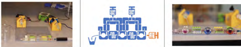
Figure 5.3: “Veggie Alchemy” experiment. From left to right: layout of the experiment with the modular blocks assembled and placed on the supporting mat; schematic of the assembly that the children have to build in order to perform the experiment; final results of the experiment, with the chromatic change achieved inside the circuit built, obtained with the modulation of the pH of the flowing solution.
