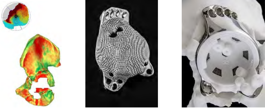
Figure 1.7: Patient specific parts for orthopedics. From left to right: image acquisition and reconstructions, 3D printed metal implant, assembly and functional implant. Adapted from materialise.com
