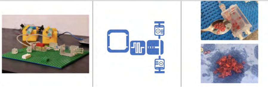
Figure 5.2: "Fruit Caviar" experiment. From left to right: layout of the experiment with the modular blocks assembled and placed on the supporting mat; schematic of the assembly that the children have to build in order to perform the experiment; final results of the experiment, with the colored alginate droplets created in the reservoir section.
