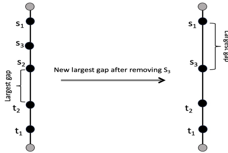
Figure 2.9: The change of largest gap and removing extra nodes in an aisle
