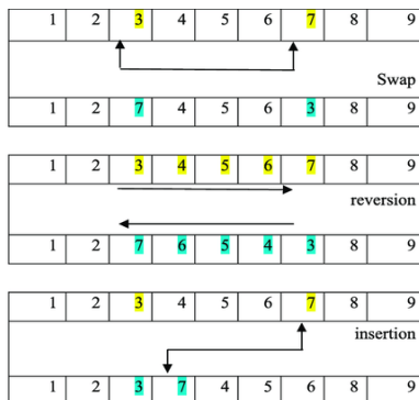
Figure 3.4: Moves considered in VNS algorithm from [119]
