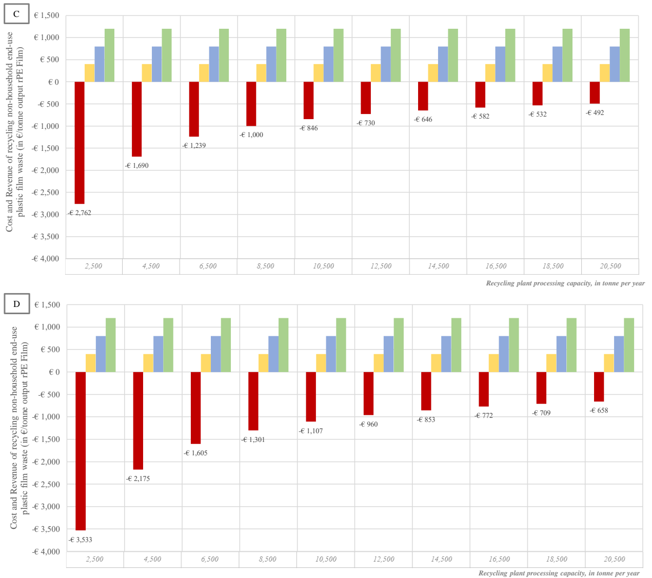
Figure D.28 Estimated annual costs (red bar) and revenue (green bar, high regranulate price; blue bar, central regranulate price; yellow bar, low regranulate price) of non-household end-use plastic film waste recycling in S1(A), S2(B), S3(C), and S4(D). The costs and revenue are shown in €/tonne rPE (y-axis) across different recycling plant processing capacity (x-axis, from 2,500 tonne/year up to 20,500 tonne/year capacity).
