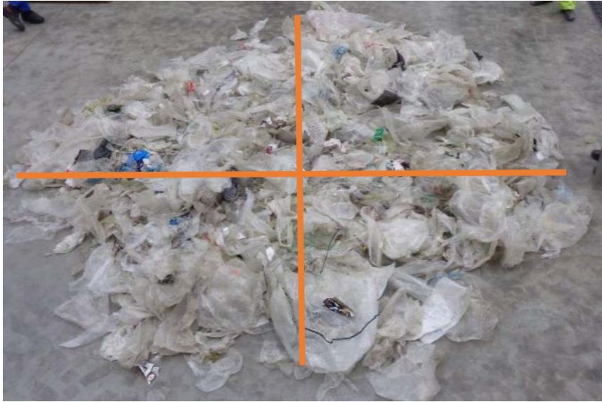
Figure C.2 Division of the output streams at each sampling point from the two randomly selected big bags that are collected at each sampling point.
