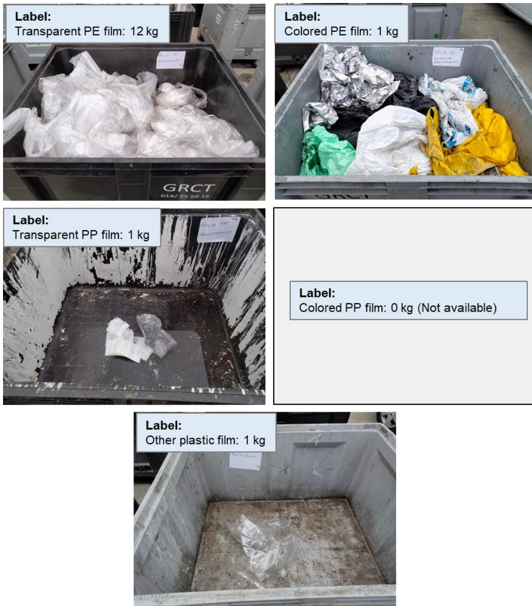
Figure D.2 Images of the collected samples from Wholesale sector (e.g., NACE sector G.46) from urban areas of Ghent.
