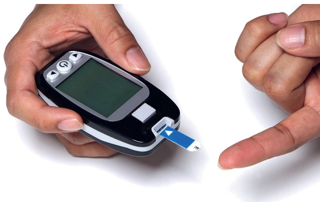
Figure 1 Representation of a commercial enzymatic glucose sensor used to measure blood glucose.[3]
