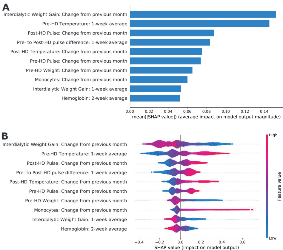
Figure 7.2 SHAP value plots for the ML model showing the extent each predictor contributes (positively or negatively) to each individual prediction. A) Bar plot of the mean absolute SHAP values for the top 10 predictors in descending order. B) SHAP value plot for the degree of the positive or negative impact of each individual measurement on the prediction (x-axis), with warmer colors representing higher observed values for that measurement, cooler colors indicating lower values for that measurement, and gray color representing a missing value for that measurement.
