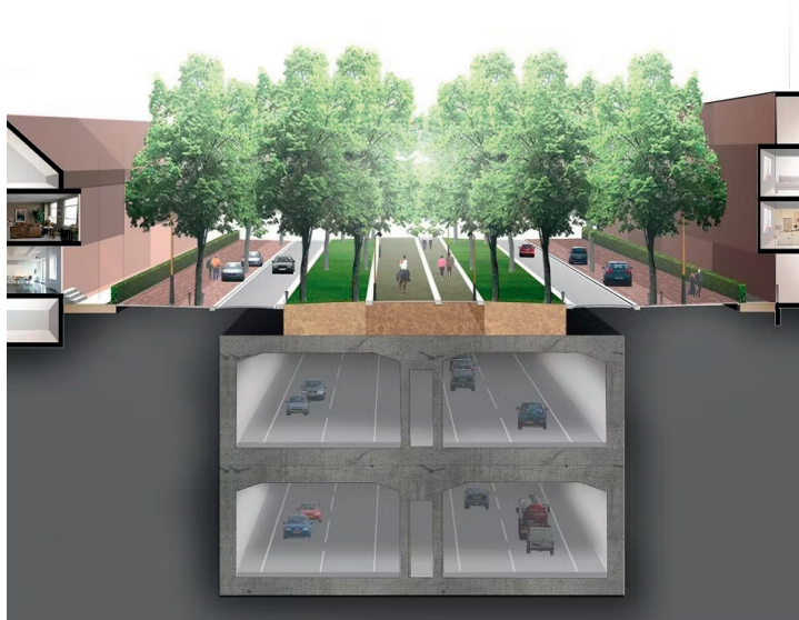
Figure 2. Schematic overview of the tunnel and the “Green Carpet” on top of it. Avenue2, ( www.a2maastricht.nl )
