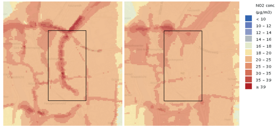
Figure 3. Nitrogen dioxide concentrations in the affected area (boxes), before the opening of the tunnel in 2015 (left) and after the opening in 2017 (right). Atlas Living Environment , ( https://www.atlasleefomgeving.nl )
