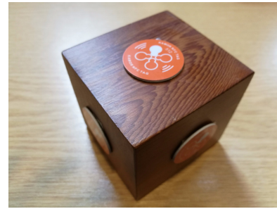
Figure 5. Alternative prototype using a wooden cube with a NFC tag on each face. The cube measures 6 cm on each side
