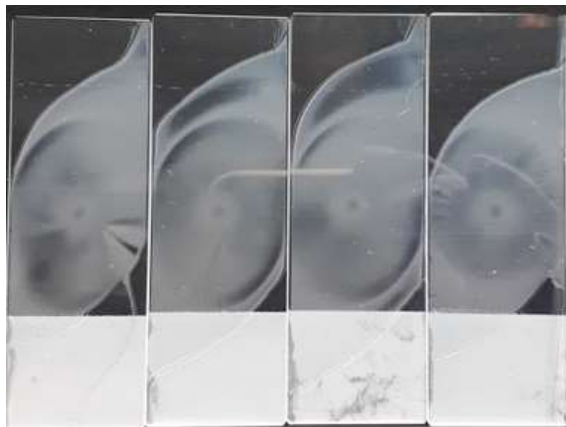
Figure A33: Spincoated microscope slides for contact angle measurement
