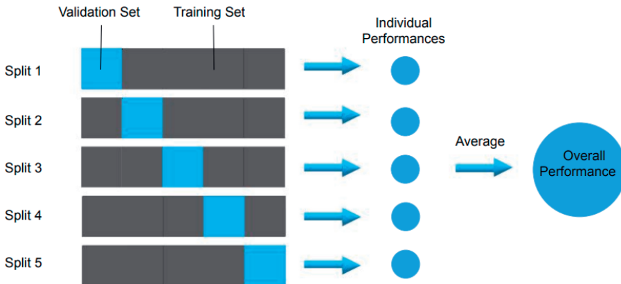
Figure 5. An example of fivefold cross-validation which can be used to evaluate machine learning models. Cross-validation gives the ability to test the result across the entirety of a dataset, giving a better estimation of a model’s overall performance.
